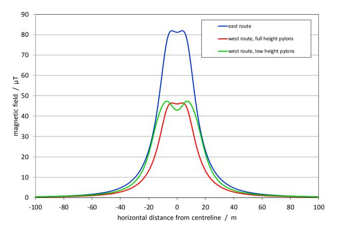
Figure 4 : Maximum magnetic fields from each proposed 400kV overhead line
