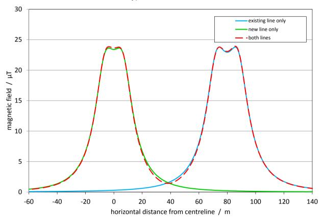
Figure 8 Combining magnetic fields from parallel overhead lines
