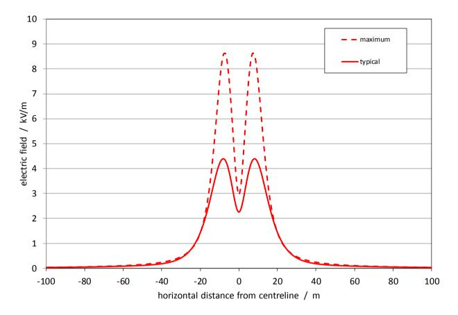
Figure 7: Typical electric fields from each proposed 400kV overhead line
