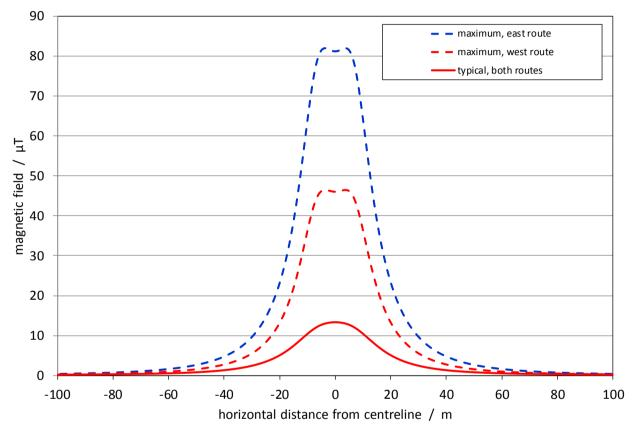
Figure 6 : Typical magnetic fields from each proposed 400kV overhead line
