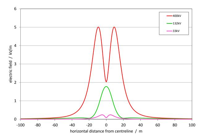
Figure 3 : Typical electric fields from existing overhead lines
