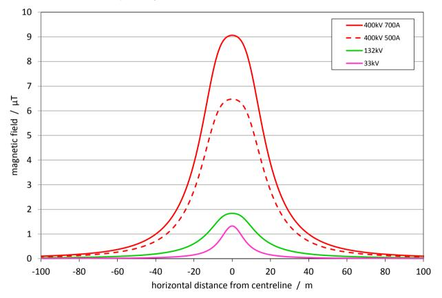
Figure 2: Typical magnetic fields from existing overhead lines
